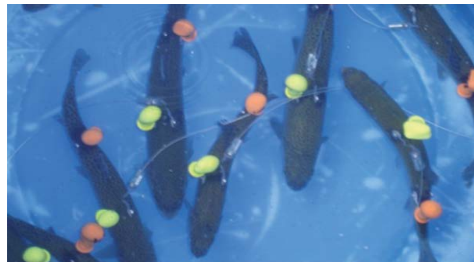
Juvenile fish (smolts) were balloon and radio tagged to validate survival and assist in redesigning and reshaping Ice Harbor Lock and Dam's spillbay #2.
